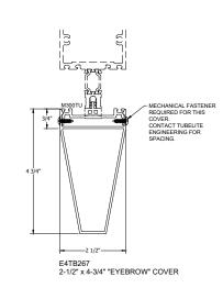
NOTE: Exterior cover profiles shown can be used for vertical application or horizontal application. Contact TUBELITE engineering for review and recommendation of attachment of covers greater 3" in depth.
