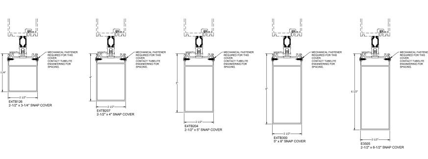
NOTE: For vertical covers greater than 5" in depth check with Tubelite engineering for suitability and review of project loads.
