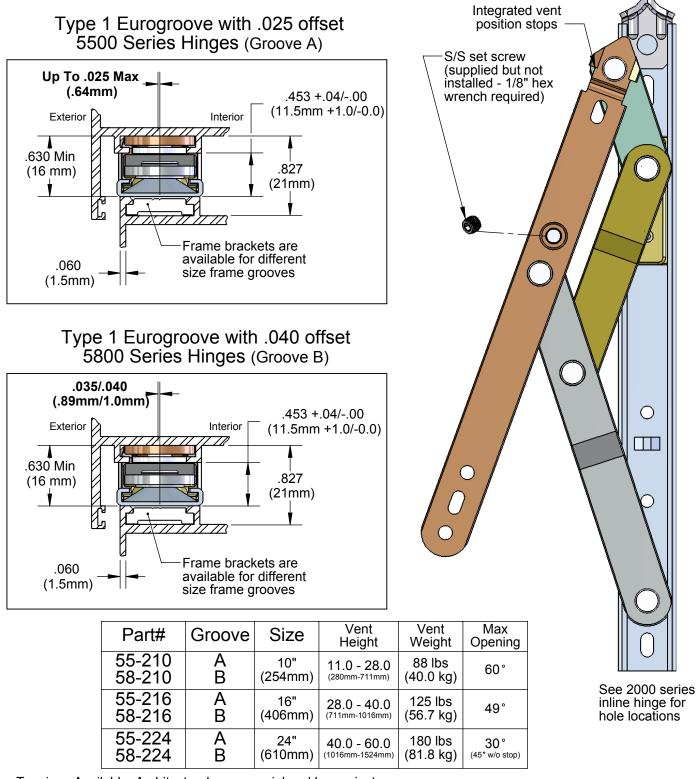
Tensions Available: Architectural, commercial and loose rivet. Hinge Mounting: Use #10 or M5 stainless steel pan head screws. Hinge Capacity: Vent size and weight should not exceed the stated capacity of the hinge. Opening Degree: For vents in high winds, severely limited opening or limited for life safety, the use of additional Limit/Friction Devices may be required (ex: 177, 419, 716).
