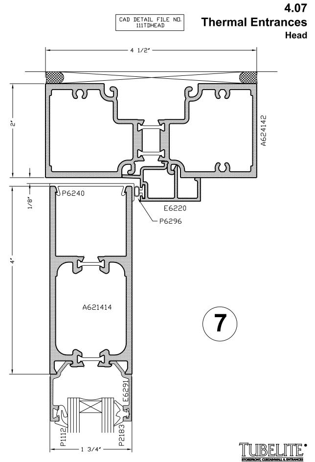
\*SEALANT, ROD, & ANCHORS NOT BY TUBELITE
