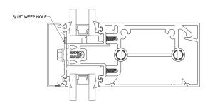
New "roll-over" shear block design: PTB110
