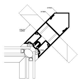
**Polyamide Pressure Plate – replaces fiberglass**
