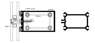
New Vertical SSG w/1/4" x 1/2" silicone structural joint (replaces 1/2" x 1/2" joint)
