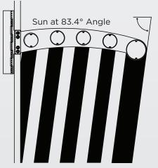
\*See Tubelite's technical manual for a complete set of Shading Table data. 25" curved outrigger with Tubular Blade shown: 30 degrees Latitude North, Summer Solstice, High Noon. Shade factor 63%.\*
