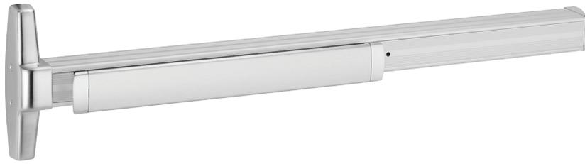
**3349A and 3549A** for hollow metal single and double doors, UL listed for panic exit hardware. Devices are ANSI A156.3 – 2008 (LBL option 2014) Grade 1. The 3549A has a smooth mechanism case and the 3349A has grooved case. The concealed vertical cable device is non-handed except when the SS (signal switch) option is used. See opposite page for available outside trim and device functions.
