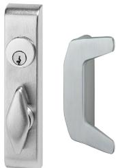
Standard operation, key locks and unlocks thumbturn. Optional operation, key unlocks thumbturn, re-locks when key is removed. This operation is created by changing the cylinder plate included with control. Use 1 1/2" mortise cylinder with a straight cam. Schlage cam reference B502-191. Not available for 3349/3549 devices.
