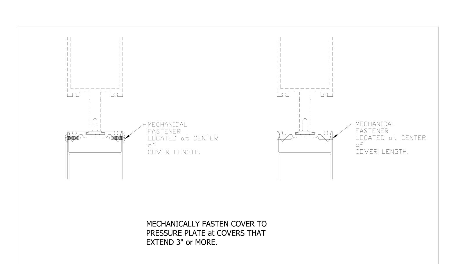
NOTE: Exterior cover profiles shown can be used for vertical application or horizontal application. Contact TUBELITE engineering for review and recommendation of attachment of covers greater 3" in depth.
