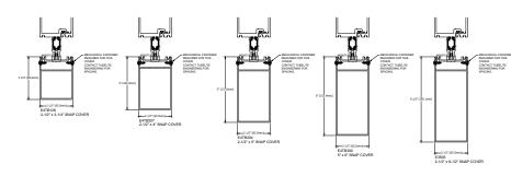
NOTE: For vertical covers greater than 5" in depth check with Tubelite engineering for suitability and review of project loads.
