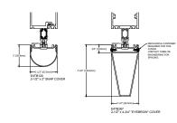
NOTE: Exterior cover profiles shown can be used for vertical application or horizontal application. Contact TUBELITE engineering for review and recommendation of attachment of covers greater 3" in depth.
