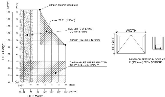
Charts are based upon an insulating glass unit infill of 1" [25.4mm] overall thickness comprised of 6mm glass/13mm gas fill/6mm glass
