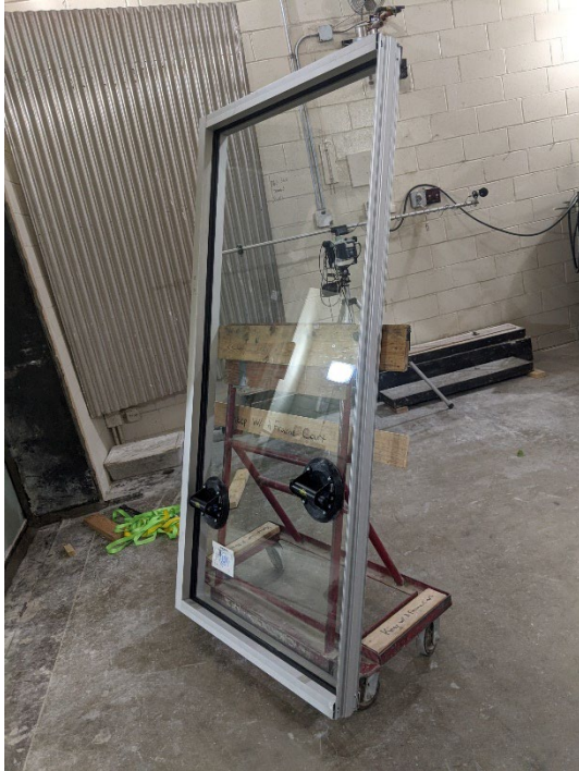
Figure 3 – One of two specimen IGUs prior to installation in test aperture
