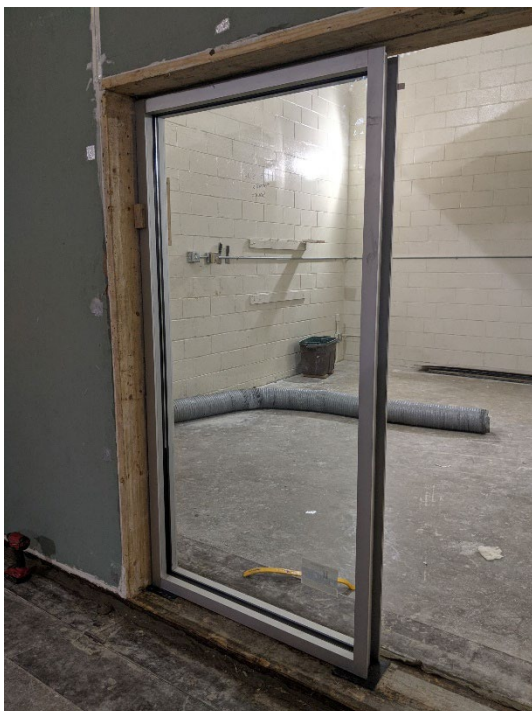
Figure 4 – Specimen partially installed in test aperture
